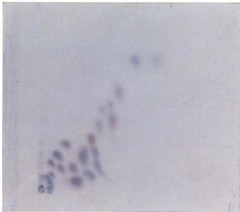
Fig. 6. Coupled-layer chromatogram of a carbohydrate mixture. Impregnation P-R; solvents 54/13.
