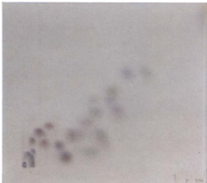
Fig. 5. Coupled-layer chromatogram of a carbohydrate mixture. Impregnation P-Q; solvents 106/13.
