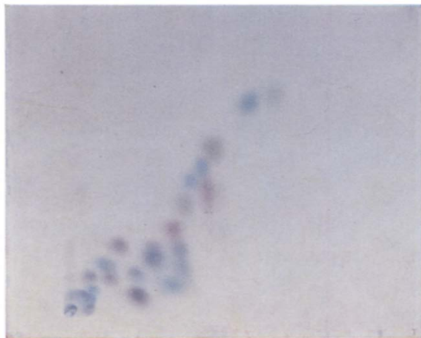
Fig. 7. Coupled-layer chromatogram of a carbohydrate mixture. Impregnation P-R; solvents 54/32.
