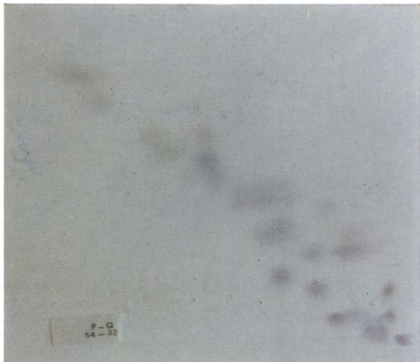
Fig. 4. Coupled-layer chromatogram of a carbohydrate mixture. Impregnation P-Q; solvents 54/32.
